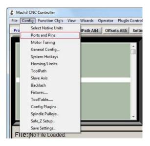
4. Enter in "Port Setup and Axis Selection" to set "Port#1" and "Kernel Speed" shown as below.
